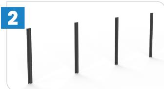
Ensure they are evenly spaced out and you have as many as required. Next, attach the hoarding panels to the posts.
