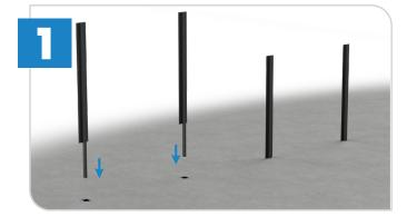
First, ensure the 2m or 2.4m posts are dug firmly in the ground, in the correct position ready for attachment.
